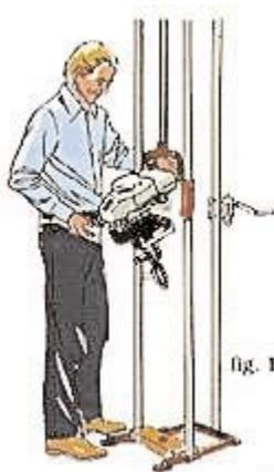
Assembly of the Power Mast takes only a few minutes and is completed by placing the engine into the cradle (fig.1).
